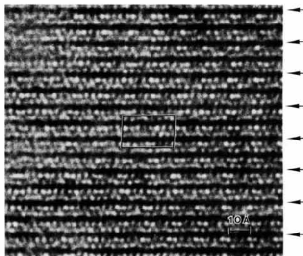
Fig. 8. A high-resolution structure image showing a [110] projection of a two-layer polytype 2M . The darkest lines running in the horizontal direction correspond to the Mn(OH)_2 sheets. Individual octahedra separated by 2.9 \text{ \AA} are imaged as dark blobs. Arrangements of white blobs corresponding to the tetrahedral sheets are identical at both sides of the octahedral sheets, indicated by arrows, proving the c axis to be doubled.
