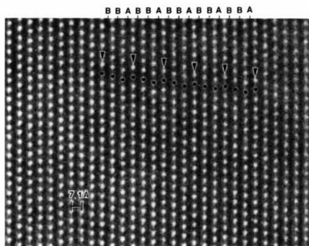
Fig. 10. A high-resolution lattice image showing a [011] projection of a three-layer polytype. A stacking sequence [022](BBA) indicated by arrows is equivalent to that of Fig. 7(b).
